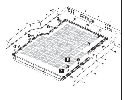
B Lift the SLIDE FLOOR up on to the vehicle's truckbed and adjust it to the center between wheel arch. (Make sure tailgate can close and the gap between slide floor's handle and the inner pamel of pick up's tailgate is 10 mm. before drilling.)
