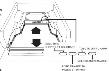
\*Always use the lower profile of truck bed as a platform to hold the SLIDE FOOR set.
